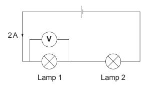
The current through lamp 1 is 2A and the voltmeter reading is 4V.
